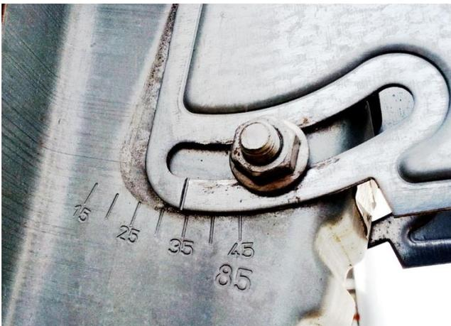
**Figure 3-1: Elevation scale markers on the antenna's mount grip**
