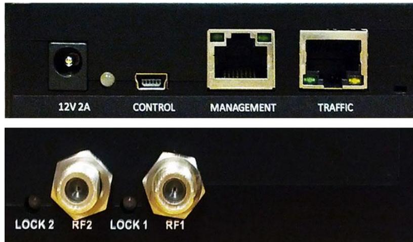
**Figure 3-3: Interfaces of DVB-S2 receiver Ayecka SR1 (top: front, bottom: back)**
